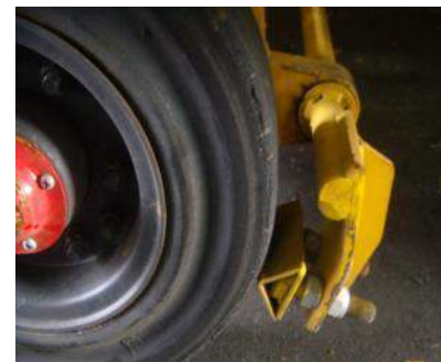
5/ Downward brake installation on dolly for safety assurance
